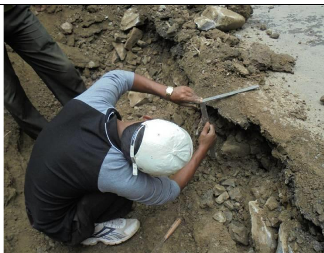
Measurement of Pavement Crust thickness at Km 95+450 on RHS
