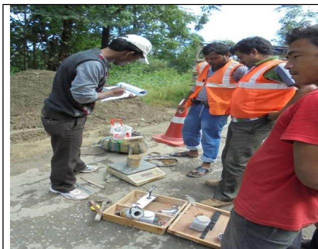
Measurement of Dry Density at Km 86+025 on LHS
