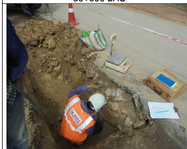
Measurement of existing crust at Km 63+150 on RHS
