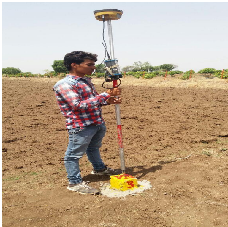
Figure 3-4 : Observation by Real Time Kinematic (GPS by RTK)
