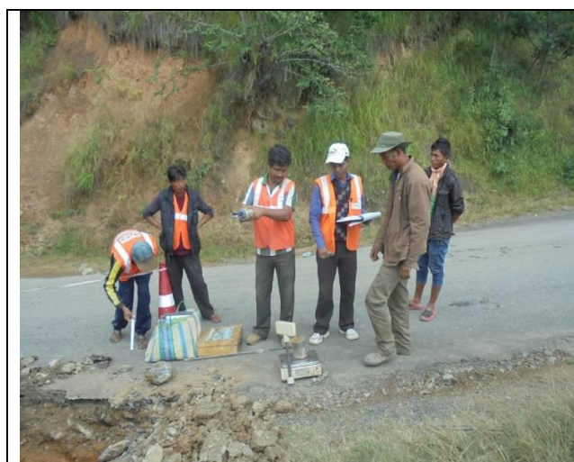
Field Dry Density Test at Km 54+140
